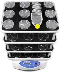
The shaker is designed for application both in small specialised laboratories and in large multidisciplinary laboratories: a choice of nine (9) different interchangeable platforms provides possibility of performing various procedures and techniques. Special attention should be paid to a multilevel platform, which allows accommodation of a large number of various microplates, Petri dishes, cultural bags and other low containers.
