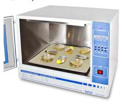
Orbital Shaker-Incubator ES-20/60 for biotechnological and pharmaceutical laboratories is a professional category equipment designed for cultivation of microorganisms and eukaryotic cells including animal, plant and insect cells. Shaker is equipped with a direct-drive mechanism for platform motion. It provides reliable and stable operation for the long term experiments needed for cell growth. Shaker-Incubator **ES-20/60** provides smooth or intensive mixing in flasks installed on the platform.
