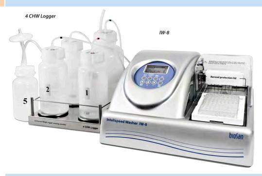
**Intelispeed Washer IW-8** is designed for washing of standard flat-bottom 96 well plates and microstrips. The unit is fully programmable ensuring multi-step solution ripening, aspiration (aspiration, combination of aspiration/liquid dispensing and soaking, as well as soaking cycle during a particular period of time).
