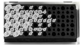
TDB-120 is a traditional Biosan's dry block thermostat for laboratory analysis. Thermostat is designed for maintaining constant temperature of samples in tubes inserted in the aluminium block sockets. Unprecedented high precision and uniformity of temperature over the block. **TDB-120** is widely used for PCR-analysis.
